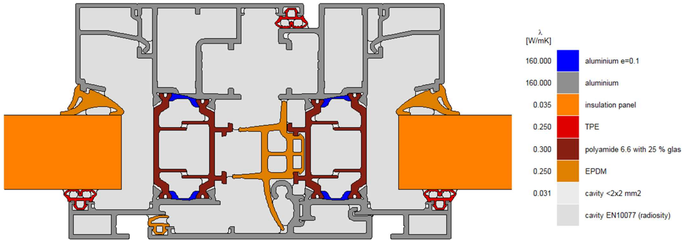
Figure 15 : Montant central – Ouvrants 011.5476.XX - 011.5477.XX+Battement 011.5480.XX+ 029.5656.04
